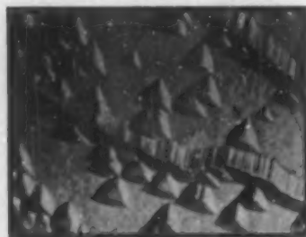
FIG. 1. Double-etch result showing dislocation motion in copper. Crystal was etched, stressed, and re-etched. 375X.
